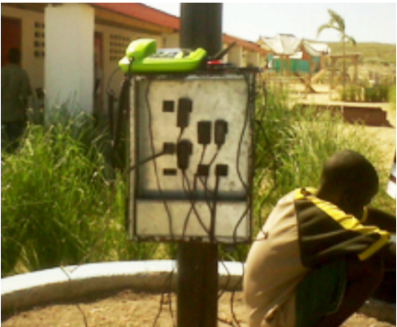
The LAMP-CELL is the latest solar street light designed and manufactured in Haiti by ENERSA. It has a cell phone charging station which can recharge 8 cell phones at the same time, up to 50 per day.
