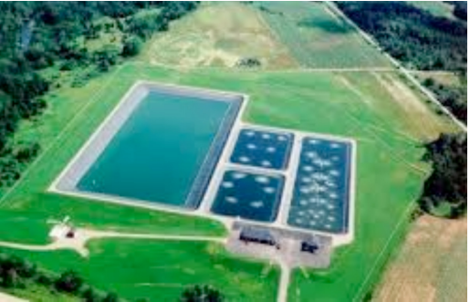
Figure 25 Aerial Image of a Partial Mix (Aerated) Lagoon (40 hectares)
