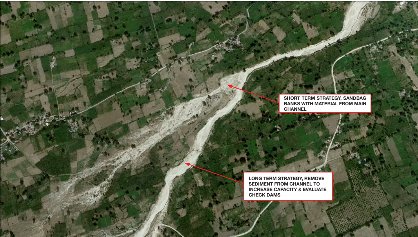
Figure 1 Major Drainage Channel Overtopping. Example of Interventions.
